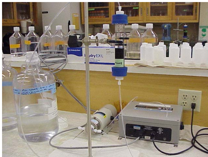
Figure 12. Laboratory GAC contact column system for Cu and Zn removal studies.
